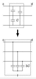
Capacitors in Delta-connection need to be transformed into equivalent Y-connection
