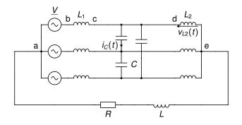
In the diagram above, it is given that  $v_a(t) = 350 \cos(\omega t + 45^\circ) V$ , with frequency f = 50 Hz,  $L_1 = 0.318 mH$ ,  $L_2 = 3.18 mH$ , C = 1.592 mF,  $R = 1 \Omega$ , L = 0.0318 mH.
