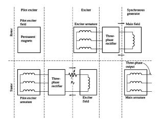
A brushless excitation scheme that includes a pilot exciter. The permanent magnets of the pilot exciter produce the field current of the exciter. Which in turn produces the field current of the main machine.
