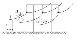
Power line model with concentrated parameters
