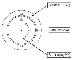
The magnetic field generated by the rotor  $B_M$  is seen by the stator winding as a varying field given by  $B = B_M \cos(\omega t)$ .
