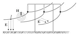
Power line model with concentrated parameters
