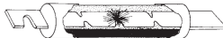
(b) The link melts and an arc is established under sustained overload current
