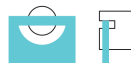
(b) Shading loop modification to pole of relay (a) for a.c. operation
