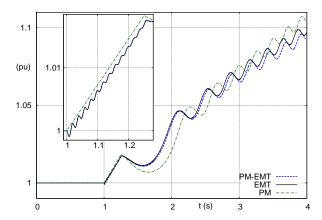
Figure 9. Case 1b: Rotor speed of generator g6
