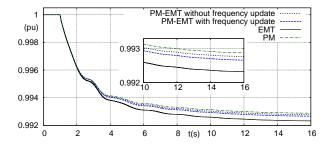
Figure 14. Case 3: Rotor speed of generator g13
