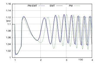
Figure 10. Case 1b: Voltage magnitude at bus 4044
