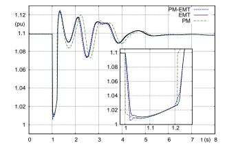
Figure 8. Case 1a: Voltage magnitude at bus 4044
