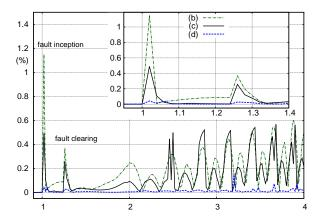
Figure 16. Case 1-b: Relative error on complex power at bus 4044 when performing a single co-simulation iteration, and using boundary conditions of types (b), (c) and (d)
