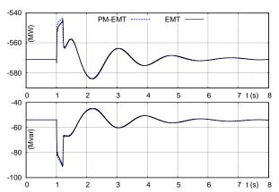
Figure 12. Case 2: active and reactive powers injected at bus 4044
