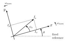
Figure 6. Reference axes involved in the phasor extraction
