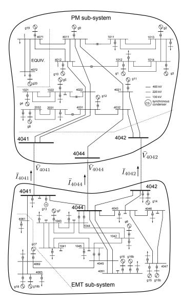
Figure 7. One-line diagram of the Nordic test system [17]
